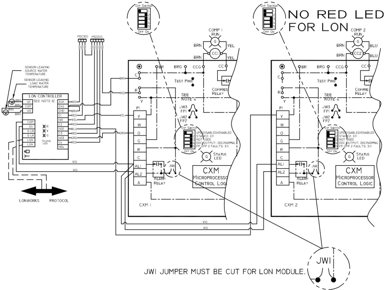
REFER TO LONWORKS INSTALLATION, APPLICATION, AND OPERATION MANUAL FOR CONTROL WIRING TO THE UNIT. LOW VOLTAGE WIRING MUST BE "CLASS I" AND VOLTAGE RATED EQUAL OR GREATER THAN UNIT SUPPLY VOLTAGE.
