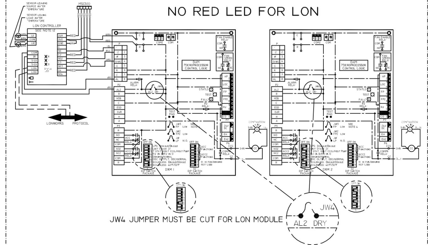
REFER TO LONWORKS INSTALLATION, APPLICATION, AND OPERATION MANUAL FOR CONTROL WIRING TO THE UNIT. LOW VOLTAGE WIRING MUST BE "CLASS I" AND VOLTAGE RATED EQUAL OR GREATER THAN UNIT SUPPLY VOLTAGE.
